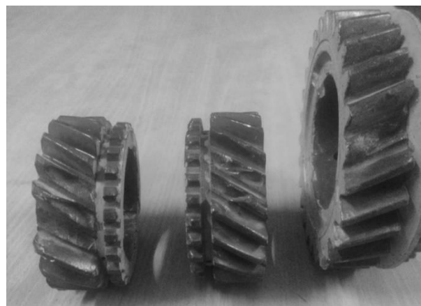
Figure 1. Fatigue failure of gear teeth.
