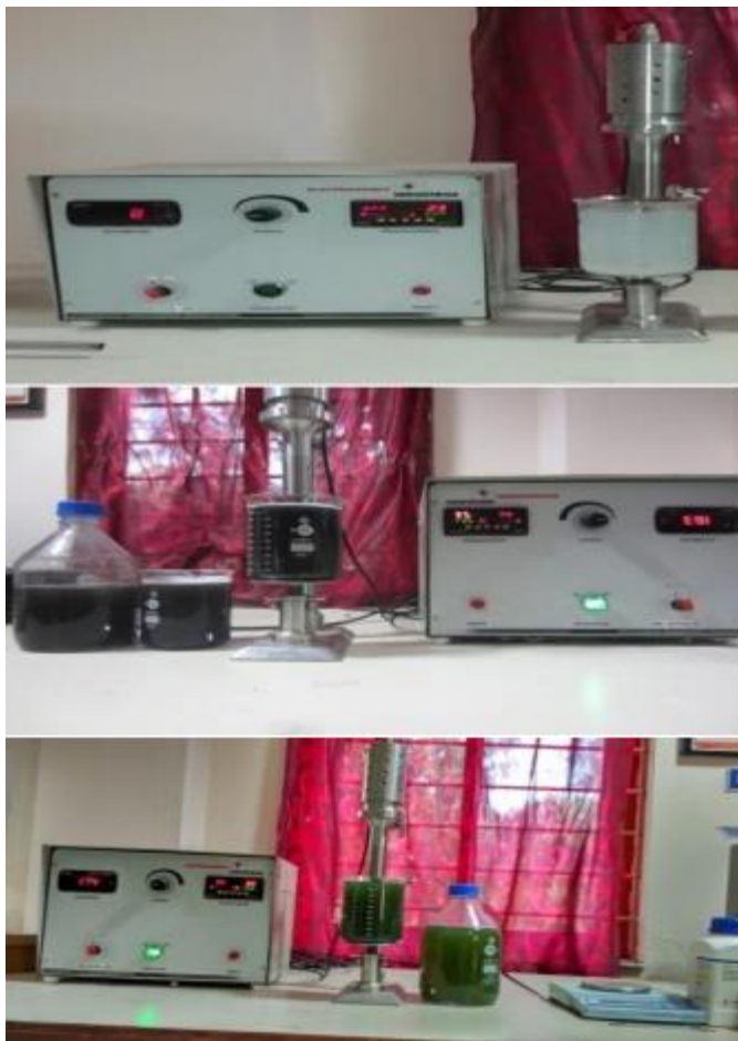
Figure 3. Using an ultrasonic sonicator to create nanofluids (i) \text{Al}_2\text{O}_3/\text{water} nanofluids.
