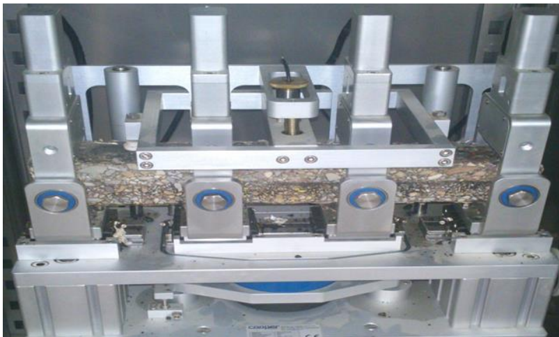
Figure 3. Dynamic Four-point flexural beam test setup.
