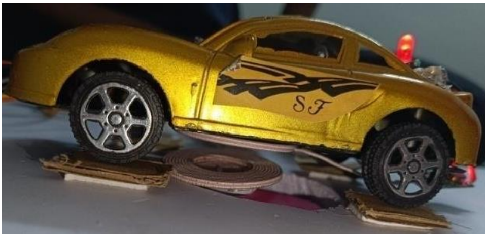
Figure 6. Transmitter and receiver coil alignment.
