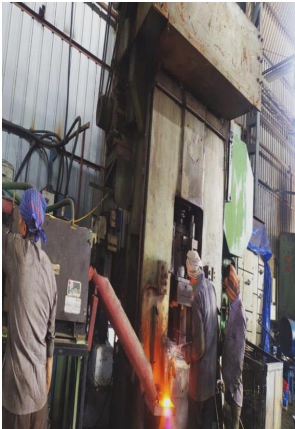
Figure 2. Mechanical screw press with automated induction heating arrangement validation and verification of experimental procedure.
