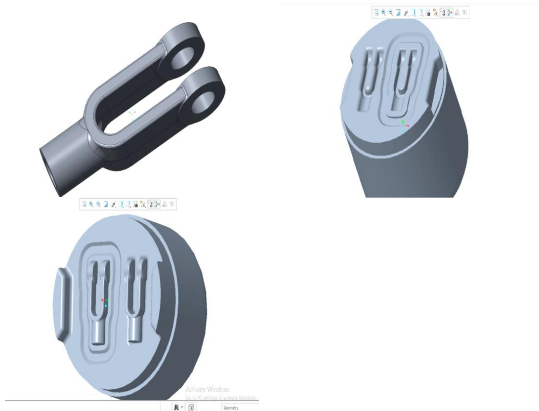
Figure 1. (a) 3D model of final machined component, (b) Die design stage.
