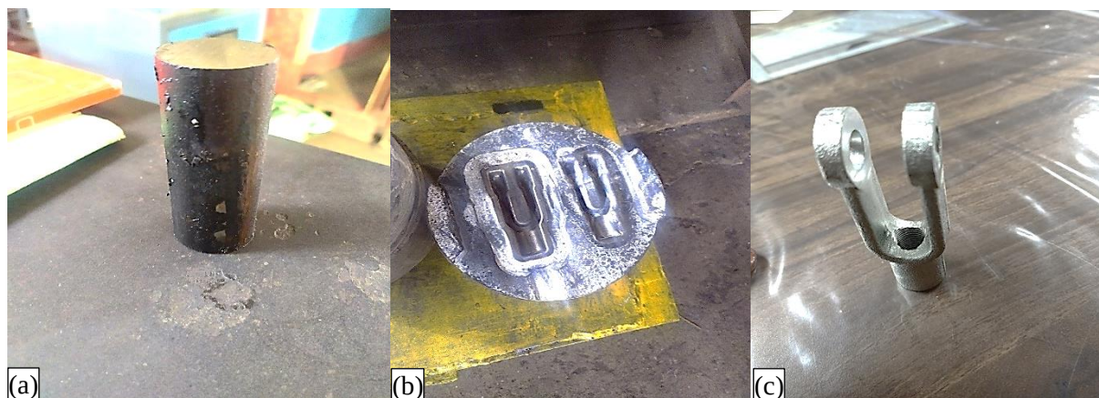
Figure 7. Actual set up showing billet and die used for experimental trial. (a) Input billet material, (b), Blocker and Finisher bottom die, (c) actual component without flash.
