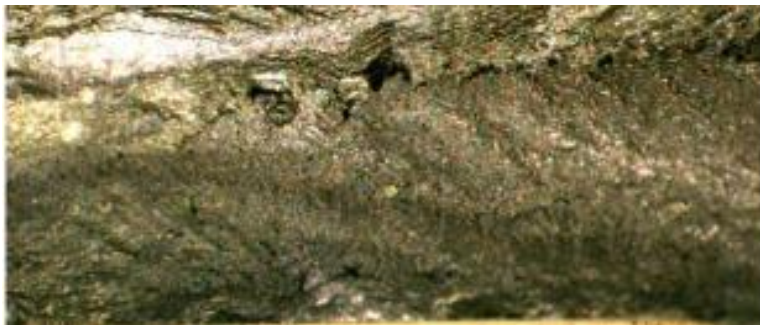
Figure 3. Topographic view of fatigue crack propagation [1].
